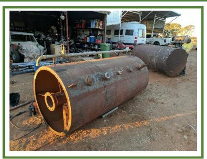
QGB have chosen to run the pyrolysis process in a kiln rather than the more traditional method of pit burning. QGB constructed the kiln themselves with a bit of research, experimentation and many hours of trial and error.
